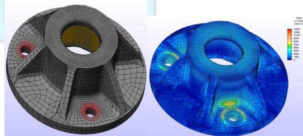
Fig. 6 FEA model of stopper under impact loading condition for determining the life of component
