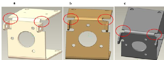
Fig. 4 Design changes in frame to reduce the stress concentration
