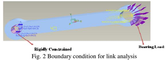
Fig. 2 Boundary condition for link analysis
