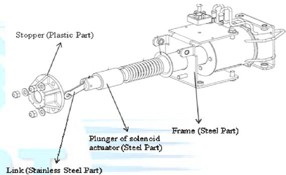
Fig. 1 Major components of stopper assembly
